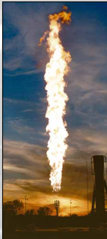
HYDRA high-performance sonic flare tip creates short, highly directional, low-radiation flames, making the HYDRA flare ideal for offshore platforms, FPSOs and other areas with limited space.
