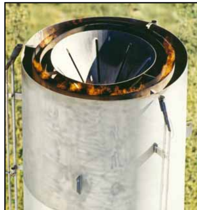
The annular swirl design of the LHLB flare prevents internal burning at low gas flow rates.
