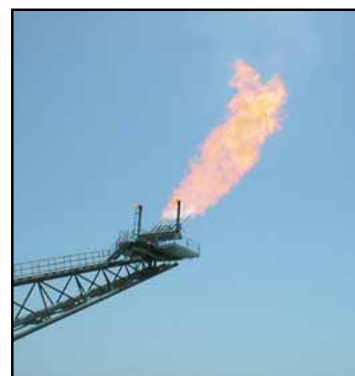
John Zink’s water injection technology produces the lowest radiation and noise levels of any high-pressure flare.
