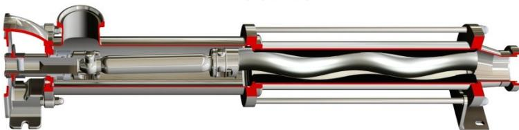
The DXO series is a hygienic pump with open joint. The design of its casing and rotating parts that are completely free of stagnation point and dead zones makes it the absolute best sanitization solution. The pin-type joint has been suitably sized to ensure a long life. Lubrication of the joint is guaranteed by the actual product thanks to its open design, consequently it is suitable for non-abrasive fluids. Performance improves considerably when pumping lubricants
