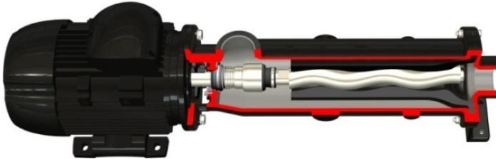
The RL series is an extremely compact product thanks to the integrated pump-electric motor construction. The patented pin joint of the Diamond series ensures high reliability. The support between the body pump and drive unit has been eliminated which makes the pump more compact and easier to maintain.
