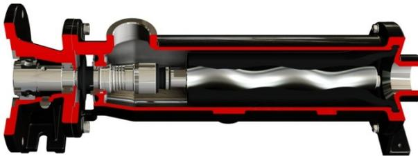
The RFL series is based on the same technology as the RL series. The difference lies in its use of a bearing housing with hollow inlet shaft. The RFL series can be connected directly to the drive with a flange. The ideal solution for the supply of a pump without a drive system, while maintaining compactness and easy installation. The bearings ensure the highest reliability in all operating conditions.
