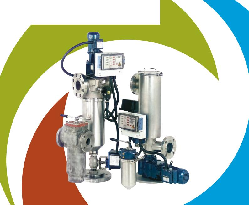
Self-cleaning filters are designed specifically to provide efficient filtration for liquids, including those of high viscosity, requiring continuous filtration without interruption to the flow during the cleaning process. There is no operator contact with the process fluid. High quality stainless steel elements are highly effective in removing contaminant particles as small as 25 micron ( $\mu$ m).
